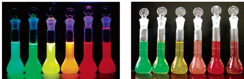
Figure 9. Size-dependent luminescence of as-prepared CdTe NCs (concentration of CdTe disperse solution was 0.4 mM, calculated by added amount of NaHTe). The emission color of TGA-stabilized CdTe NCs can be adjusted by their size to be cyan, green, yellow, orange, red, and dark red under the radiation of the UV lamp (left). The colors of the samples were also observed in sunlight (right).
