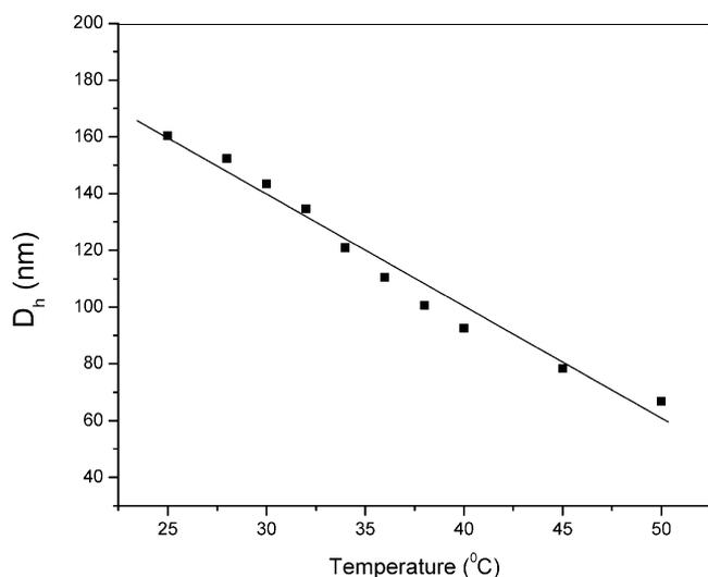
Fig. 2. The influence of temperature on hydrodynamic diameter of the PSI-PA-3 (DS=70%) aggregates in water medium (Detected angle: 90°).
