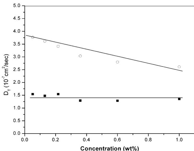
Fig. 5. Diffusion coefficient  $D_T$  of PSI-PA-3 (DS = 70%, ○) aggregates and PDDA-PA-4 (DA:PA = 48:52 ■) in water solution as a function of the concentration (detected angle: 90°, temperature: 25 °C).
