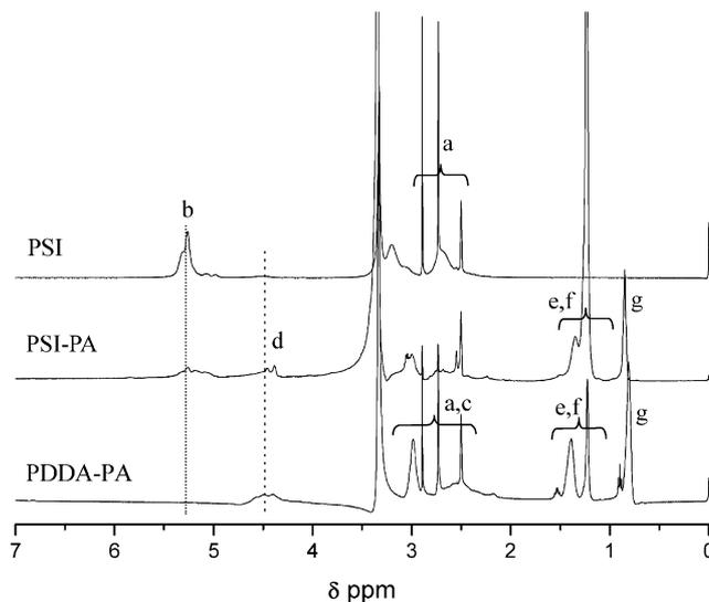
Fig. 1.  $^1\text{H}$  NMR spectra of PSI, PSI-PA (DS=76%) and PDDA-PA (DPA/PA=24:76) in  $\text{DMSO}-d_6$  at  $25\text{ }^\circ\text{C}$ .
