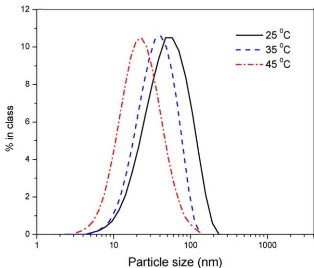
Fig. 3. Size distribution of PDDA-PA-4 (DDA:PA=48:52) in 0.25% aqueous solution at different temperatures.
