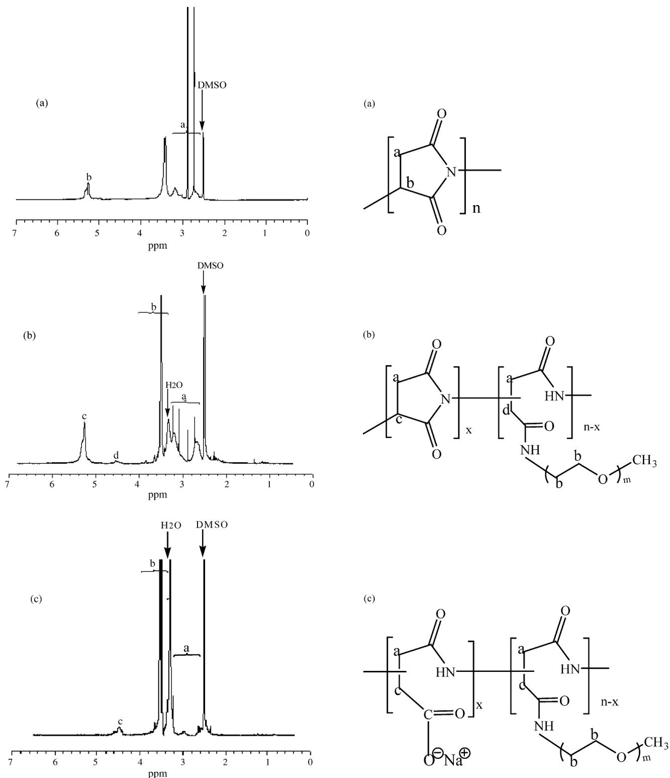
Fig. 1.  $^1\text{H}$  NMR spectra of PSI (a), PEG-g-PSI (b) and full-opened PEG-g-PAsp (c).
