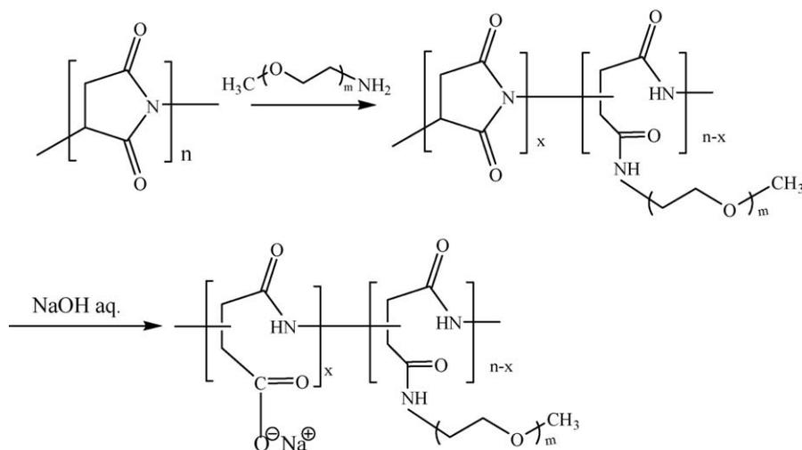
Scheme 1. The overall synthetic route of poly(ethylene glycol)-grafted poly(aspartic acid) (PEG-g-PAsp).
