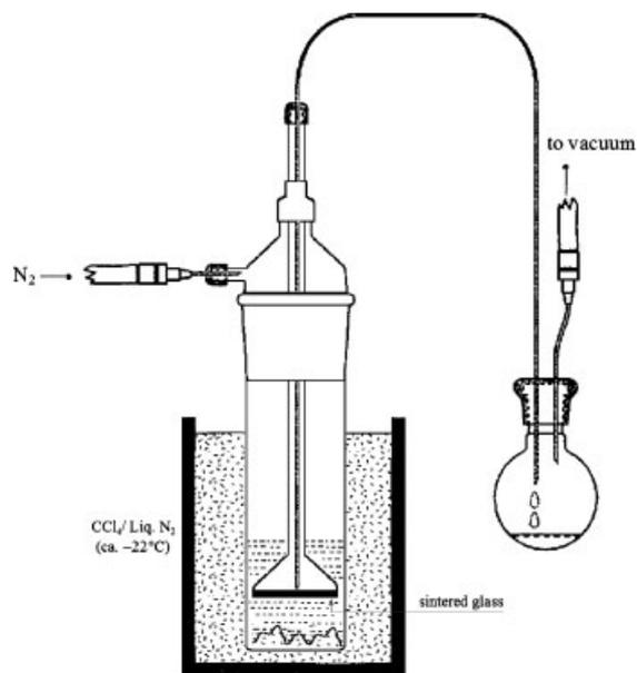
**Figure 2.** The general assembly for recrystallization of the polymerizable amphiphiles at low temperature and in nitrogen atmosphere.
